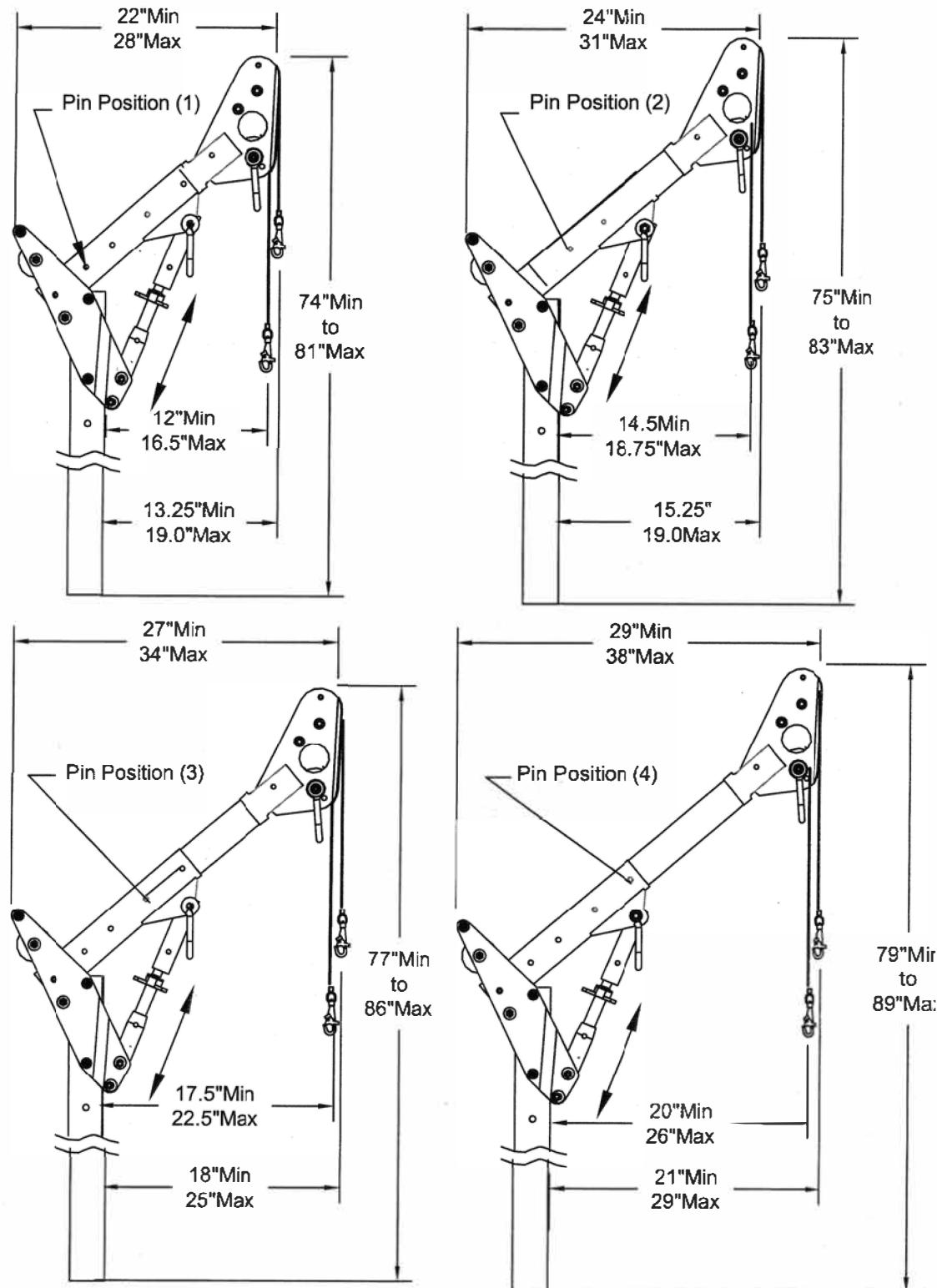
**\*MAXIMUM OFFSET DETERMINED WITH ADJUSTABLE GUSSET FULLY COLLAPSED (NO VISIBLE THREADS)**
